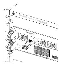
Figure 16: Installing an XFP Module (Summit family switch and BlackDiamond 8800 series switch)
